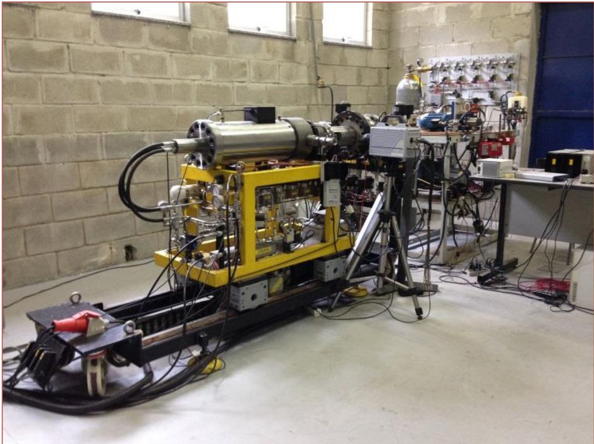
Figure 2. RCM installed on VEL at PUC – Rio.
